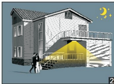
2 With insufficient daylight,even when motion detected.light ON.
